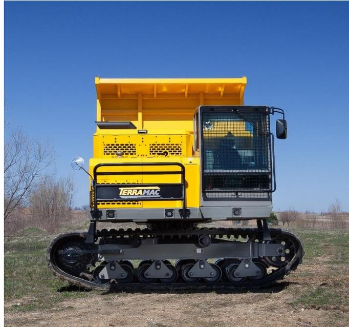
Photo Caption 2: The new Terramac RT14R crawler carrier is equipped with a rotating upper frame to provide superior productivity and reduced cycle times.
