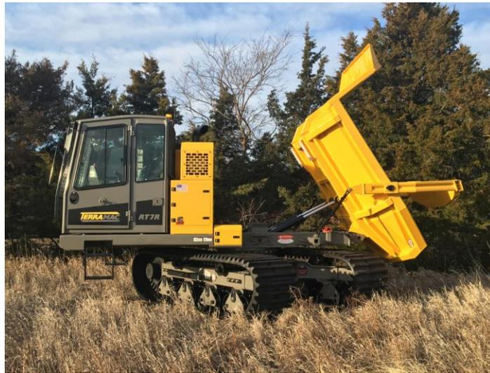
Photo Caption 2: The new Terramac RT7R can carry and dump up to 14,000 lbs. of material at any position, even while driving.
