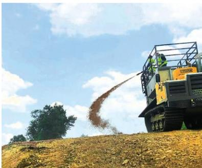
Photo Caption 1: Terramac RT9 applying the ADC slurry.
